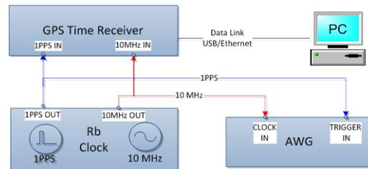
**Figure 5. Clock Monitoring with a GPS Time Receiver**
