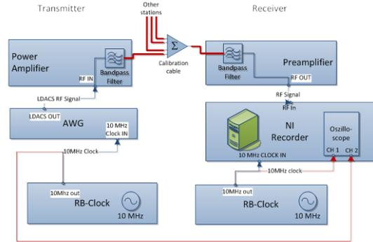
**Figure 7. Calibration Setup for a Single Station**
