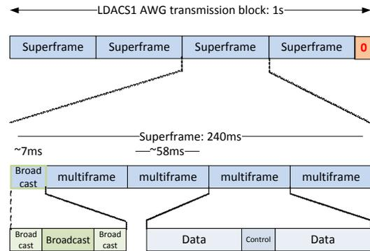
Figure 8. Structure of the Transmitted LDACS1 Signal
